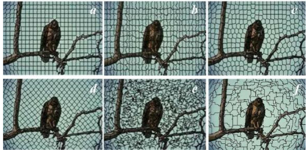
Figure 1. The six typical superpixel segmentation results. (a) SLIC [6], (b) PB [14], (c) LSC [8], (d) DBSCAN [11,12], (e) ERS [9], (f) SEEDS [13].
