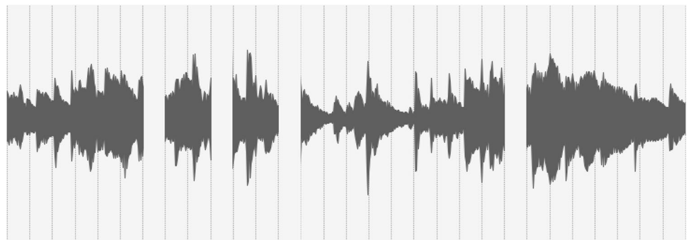
Fig. 4 Visual representation of 10% packet loss in a waveform
