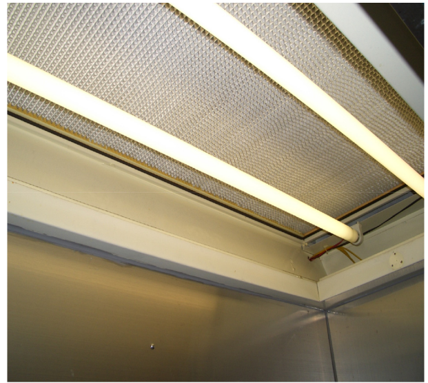
Fig. 1. Example of the faulty design of biosafety cabinets due to the fluorescent light, which was disturbing the tests for the downflow velocity and efficiency of the HEPA filters. HEPA, high efficiency particulate air.
