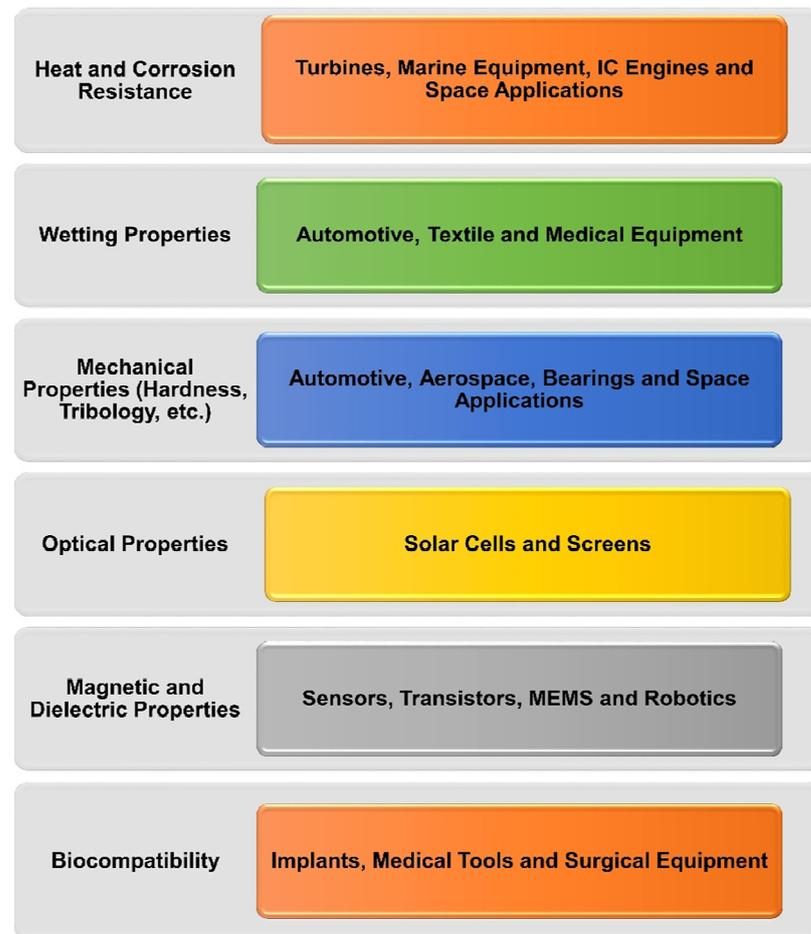
**Figure 19.** Application areas of nanostructured coatings [225].
