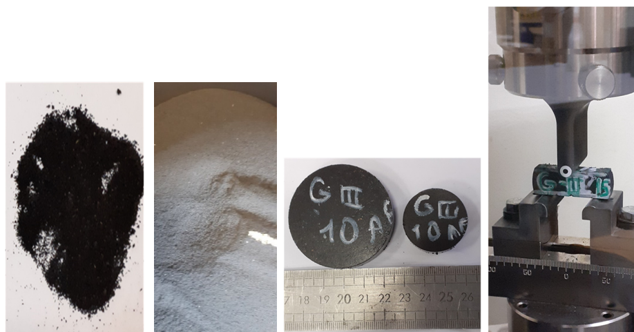
Three-Point single edge (3PB-SENB) notch bending test device
