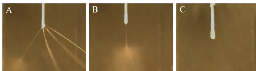
Figure 2. Three working modes of electrospinning process: (A) multi-jet mode ( V = 6 kV, Q = 30 \mu L/min, Z = 30 mm), (B) single-jet mode ( V = 4.5 kV, Q = 30 \mu L/min, Z = 30 mm), and (C) dripping mode ( V = 3.5 kV, Q = 30 \mu L/min, Z = 30 mm).
