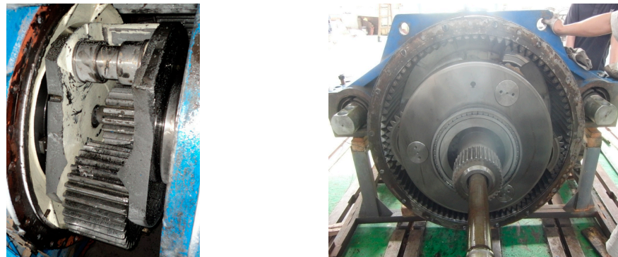
Figure 19. Damaged wind turbine gearbox due to planet gears failure.
