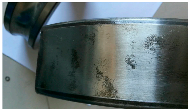
Figure 17. Scuffing on the outer race of a generator bearing due to looseness.
