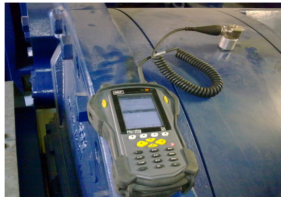
Figure 7. Portable data acquisition system for wind turbine drivetrain.
