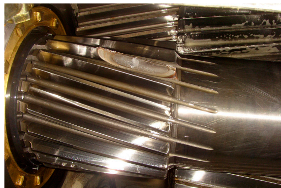
Figure 13. Broken pinion on high-speed shaft of a wind turbine gearbox.
