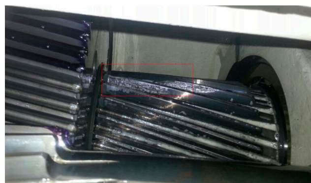
Figure 10. Chipped pinion on intermediate shaft of a wind turbine gearbox.
