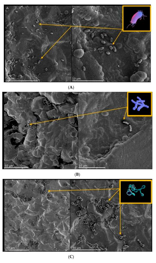
**Figure 5.** Colonization of the tested biomaterial (Ti/TiN + 7.5% Ag) by microorganisms (bacteria and fungi). Surface morphology (SEM) with the: (**A**) *Pseudomonas aeruginosa*, (**B**) *Streptococcus pyogenes*, (**C**) *Candida albicans*.
