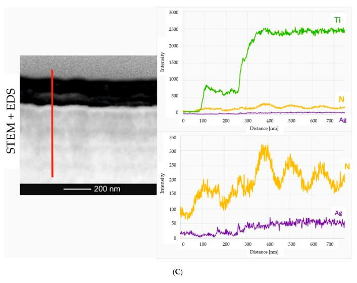
Figure 2. TEM/BF and HREM images of distribution of Ag nanocrystallites in  $Ti/Ti_2N$  multilayer (**A**), STEM image and accompanying maps presenting distribution of Ti, N, Ag, C elements from area marked with square (**B**) and profiles of chemical composition across the multilayer (along the marked line) (**C**).
