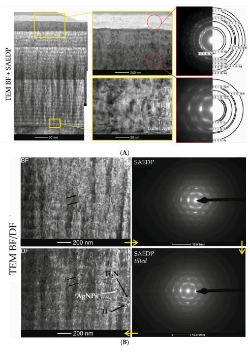
Figure 1. TEM/BF images and accompanying electron diffractions: (A) of multi-layer  $\text{Ti/Ti}_X N$  coating with thickness (~3.80  $\mu$ m) implanted with Ag nanoparticles (12.5% at.), (B) of Ag nanocrystallites in both Ti and  $\text{Ti}_2 N$  layers.
