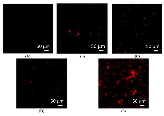
**Figure 6.** The viability of bacteria on the surface of the tested biomaterials. **(A)** Reference substrate, **(B)** Ti/TiN + 5% Ag, **(C)** Ti/TiN + 7.5% Ag, **(D)** Ti/TiN + 10% Ag, **(E)** Ti/TiN + 15% Ag.
