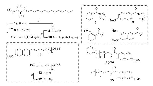
**Scheme 1.** Synthesis of sphingolipid benzoyl and (6-methoxy-2-naphthoyl) derivatives. *a*, EDCI, DMAP, 6-methoxy-2-naphthoic acid, CH<sub>2</sub>Cl<sub>2</sub>; *b*, *N*-benzoylimidazole (**5**), DBU, CH<sub>2</sub>Cl<sub>2</sub>; *c*, H<sub>2</sub> (1 atm), 10% Pd-C, EtOAc; *d*, *N*-(6'-methoxy-2'-naphthoyl)imidazole (**9**), DBU, CH<sub>2</sub>Cl<sub>2</sub>.
