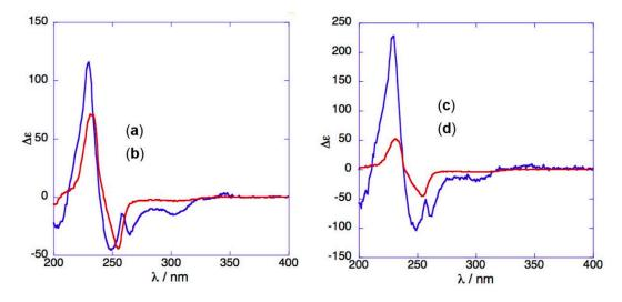
**Figure 3.** CD spectra (23 °C) of (a) (red) *N*,*O*,*O*'-tri-(6'-methoxy-2'-naphthoyl)-D-sphingosine (8) in MeOH ( $c = 1.4 \times 10^{-5}$  M) and (b) (blue) 8 in DSPC liposomes ( $c = 5.87 \times 10^{-5}$  M); (c) (red) *tris*-(6'-methoxy-2'-naphthoyl)-D-sphinganine (10) in MeOH ( $c = 1.4 \times 10^{-5}$  M) and (d) (blue) 10 in DSPC liposomes ( $c = 1.4 \times 10^{-5}$  M).
