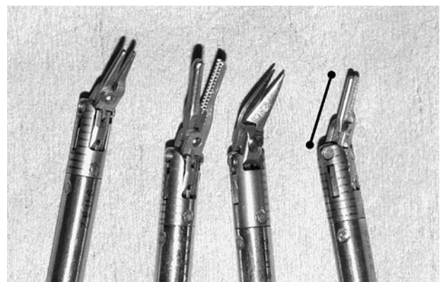
Fig. 2 Zeus “MicroWrist” robotic instruments. This is a small sample of available Zeus robotic instruments. This study used the micro-needle holder shown at the far right , with a jaw length of 7 mm, and overall “hand” length of 11 mm ( line )
