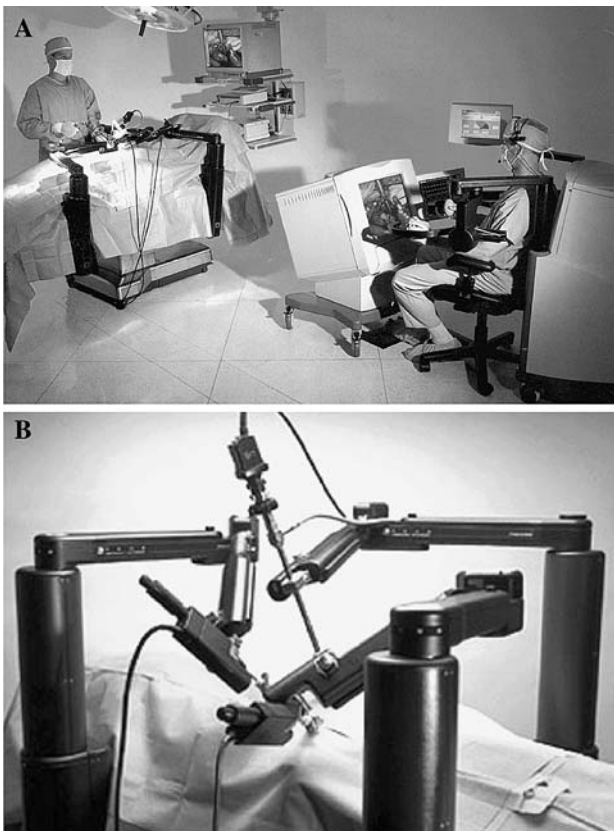
Fig. 1 Zeus surgical robot. a Zeus surgical telemanipulator system. Surgeon sits at control console at right, with control unit behind, and three monitors in front. The large monitor furnishes a high-resolution two-dimensional endoscopic view of the surgical workspace; the next monitor to the right shows Hermes voice-commands for the Aesop camera holder; the third monitor shows motion-scaling and other details of robotic control. b Robotic instrument arms and Aesop endoscope arm (not sterile-draped) at the operating table
