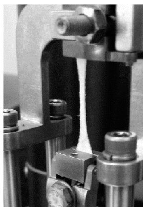
Figure 9. The nonwoven sample temporary shape in the clamps DMA apparatus.
