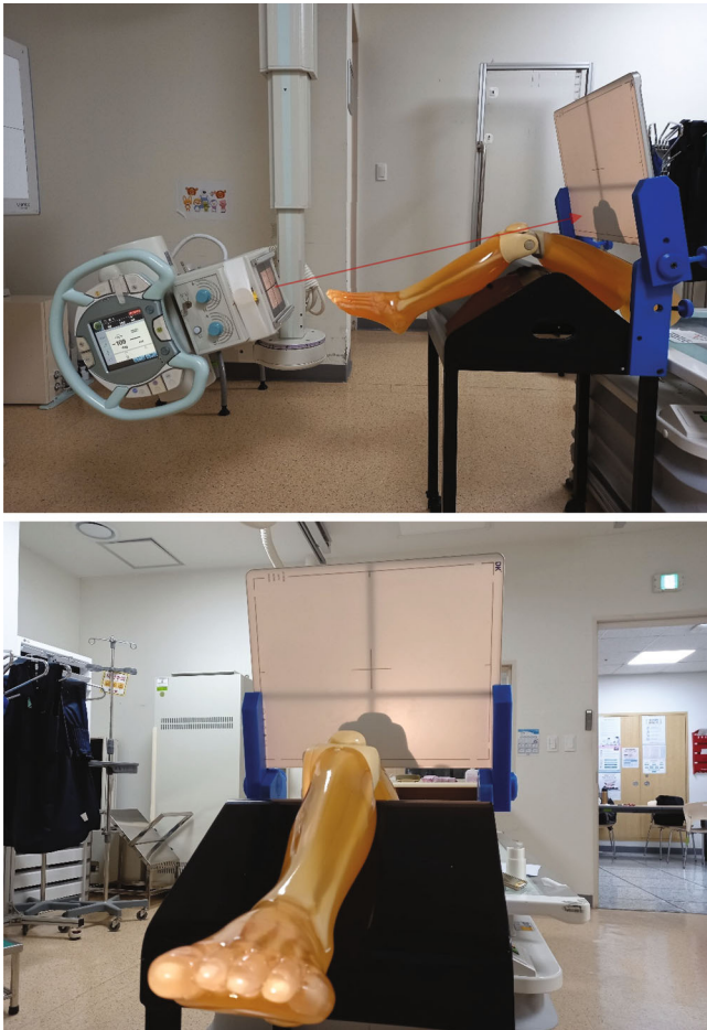
FIGURE 4: A phantom was mounted on the developed body of the PJR, and radiographs were taken in the tangential axial projection.
