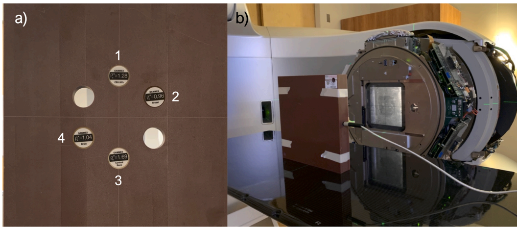
Fig. 3. a) In-house contrast phantom containing 1) CB2-30% 2) breast 3) cortical bone 4) brain tissue equivalent inserts and two voids for additional materials and b) thin contrast phantom imaging setup at 98 cm SSD.
