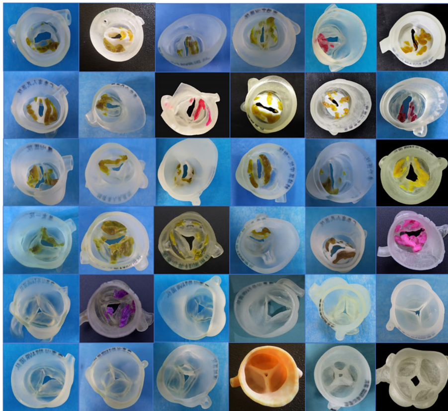
Fig. 2 Multicolor and multimaterial 3-dimensional printed models of aortic roots with different types of leaflets (leaflets as soft materials; calcifications as hard materials)
