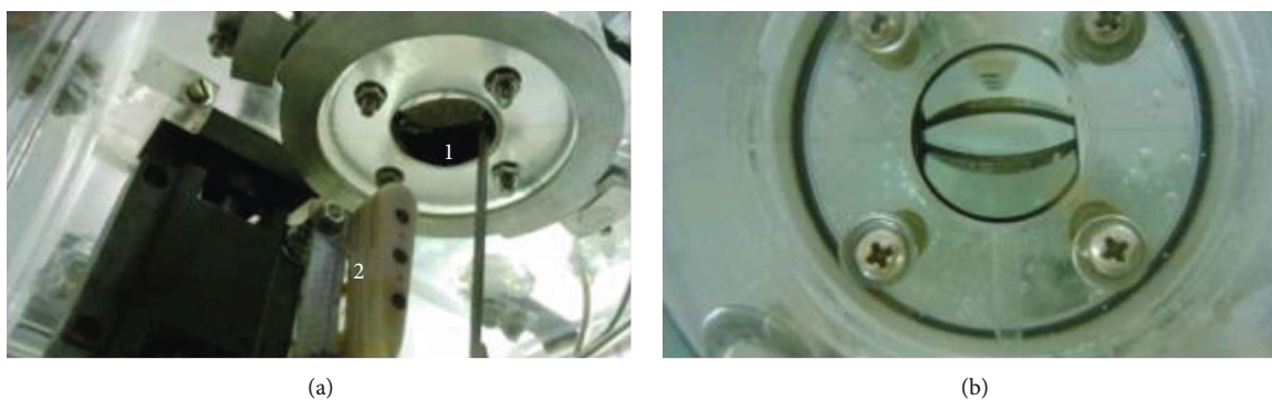
FIGURE 4: Location of the pressure sensors downstream of the open bileaflet valve.
