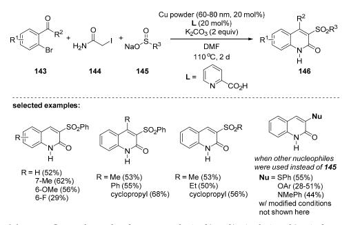
Scheme 42. Cu-powder-catalyzed one-pot synthesis of 3- and/or 4-substituted 2-quinolones.
