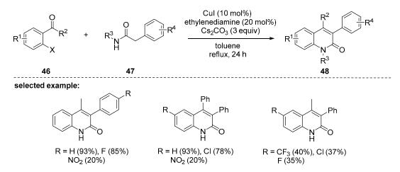
**Scheme 12.** Copper iodide-catalyzed synthesis of 2-quinolones via cascade reactions of 2-halobenzocarbonyls with 2-arylacetamides.
