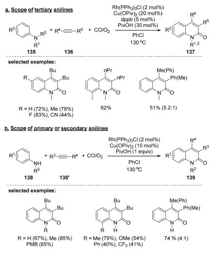
Scheme 40. Rh-catalyzed aerobic oxidative cyclization of simple anilines with internal alkynes.
