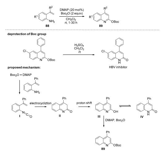
Scheme 26. DMAP-catalyzed cyclization of Boc-anhydride of 2-alkenylanilines.
