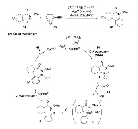
Scheme 18. Rh-catalyzed synthesis of 3,4-cycloalkaquinolones using N-alkoxyamides and boronic esters.
