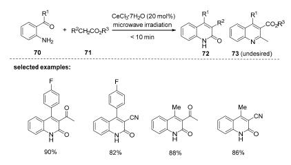
**Scheme 20.** Microwave-assisted, solvent-free synthesis of substituted 2-quinolones by reaction of *o*-aminoarylketones with esters.
