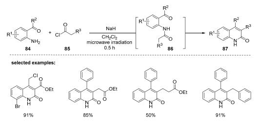
**Scheme 25.** Synthesis of 3,4-disubstituted 2-quinolones by one-pot condensation promoted by microwave irradiation.
