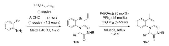
Scheme 45. Preparation of 2-quinolones using four-component adduct via Heck reaction.
