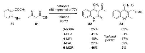
Scheme 24. Friedländer reaction by bifunctional zeolites as Lewis and Brønsted acid catalyst.
