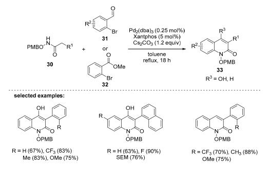
**Scheme 7.** Synthesis of *N*-hydroxyquinolin-2(1*H*)-ones through a sequential Buchwald-type amidation/cyclization process with PMB (*p*-methoxybenzyl)-protected *N*-hydroxyamides.
