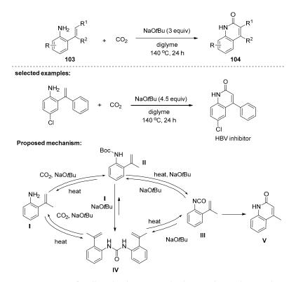
Scheme 30. Lactamization of 2-alkenylanilines toward substituted 3,4-substituted 2-quinolones.
