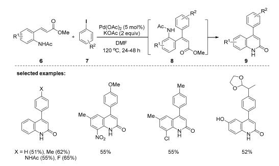
**Scheme 2.** Synthesis of 4-aryl-2-quinolones through a sequential Heck reaction cyclization of methyl- $\beta$ -(2-acetamidoaryl)acrylates **6** and aryl iodides **7**.
