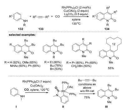
Scheme 39. C-H activation of anilines with alkynes and CO gas.
