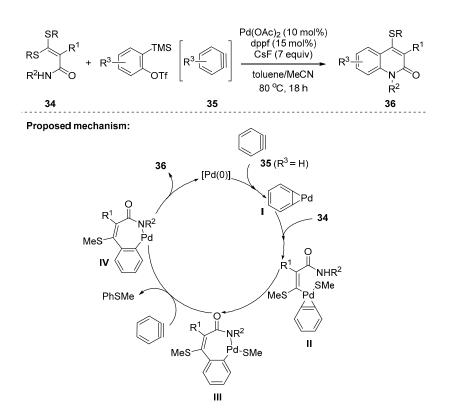
**Scheme 8.** Synthesis of 2-quinolinones by Pd-catalyzed C–S activation/aryne insertion/intramolecular C–N coupling reaction.
