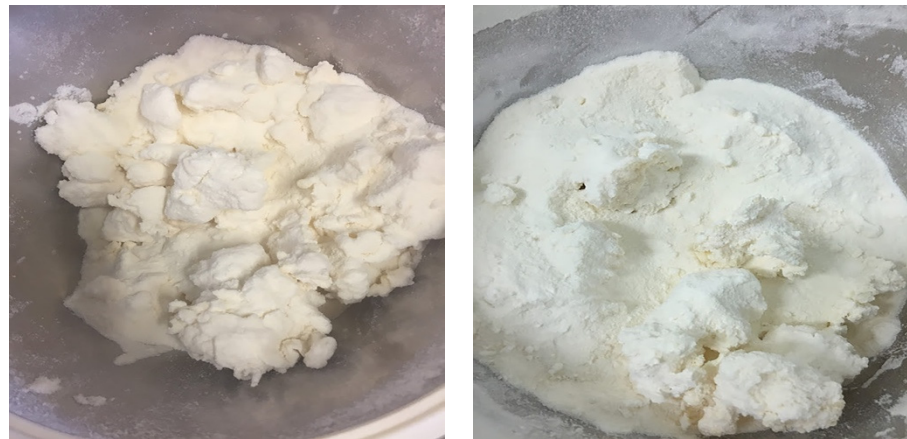
Figure 3. The resultant agglomerated powder in treatments that had the combination of 140 g pre-wet mass and 5.6 mL·min -1 flow rate. The resultant powder did not meet the industrial specification of WPI.
