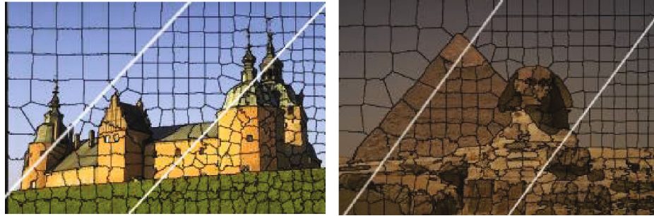
FIGURE 7: Result of segmenting 100, 300, and 500 superpixels with the SMBFT method.
