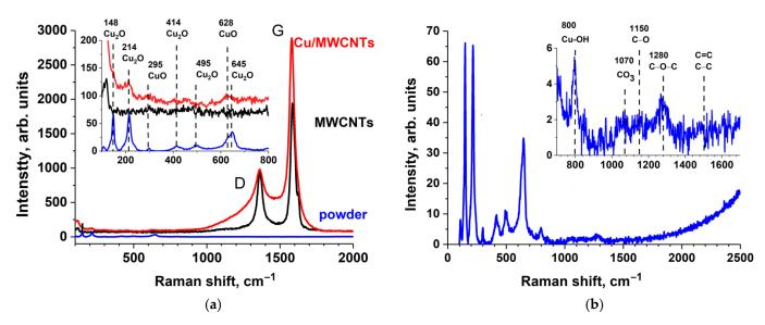
**Figure 6.** Raman spectra of (**a**) the initial MWCNTs, Cu/MWCNTs hybrid nanocomposite, and (**b**) powder from the reactor walls formed during the composite synthesis.
