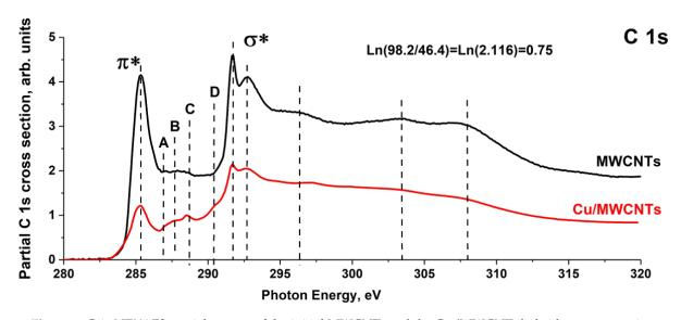
Figure 7. C 1s NEXAFS partial spectra of the initial MWCNTs and the Cu/MWCNTs hybrid nanocomposite.
