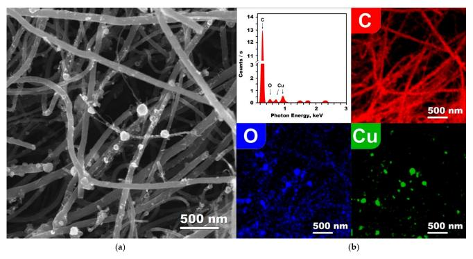
**Figure 5.** (a) SEM image and (b) EDS data of the Cu/MWCNTs hybrid nanocomposite: EDS spectrum and maps of spatial distribution of carbon, oxygen, and copper atoms.
