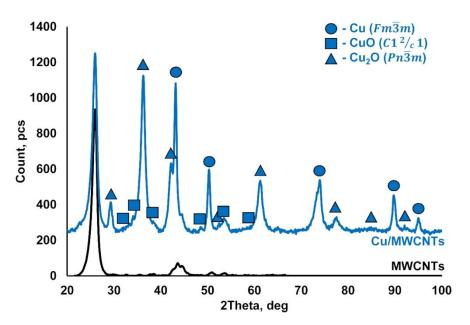
**Figure 3.** Powder XRD patterns of the initial MWCNTs (black) and Cu/MWCNTs hybrid nanocomposite (blue).
