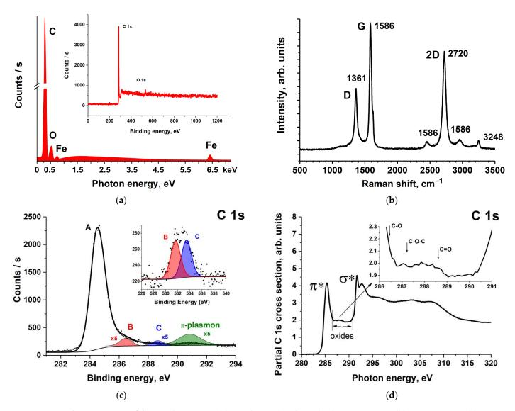
**Figure 2.** Characterization of the initial MWCNTs: (a) EDS (bottom) and XPS (top) survey spectra, (b) Raman spectra, (c) C 1s and O 1s XPS spectra, and (d) C 1s NEXAFS spectrum.
