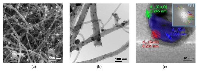
**Figure 4.** Electron microscopy images of the Cu/MWCNTs hybrid nanocomposite: (a) SEM; (b) TEM; (c) HRTEM of a lonely nanotube with the FFT pattern in insert.
