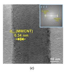
**Figure 1.** Electron microscopy images of the initial MWCNTs: (a) SEM; (b) TEM; (c) HRTEM of a lonely nanotube with the FFT pattern in insert.
