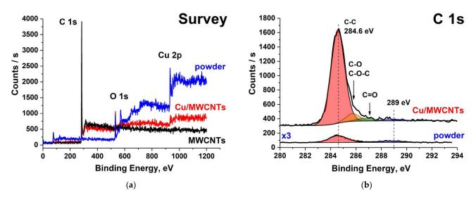
**Figure 8.** XPS spectra of the initial MWCNTs, Cu/MWCNTs hybrid nanocomposite, and powder from the reactor walls: (a) survey and (b) for the C 1s. The intensity of the powder C 1s spectrum was increased by 3 times.
