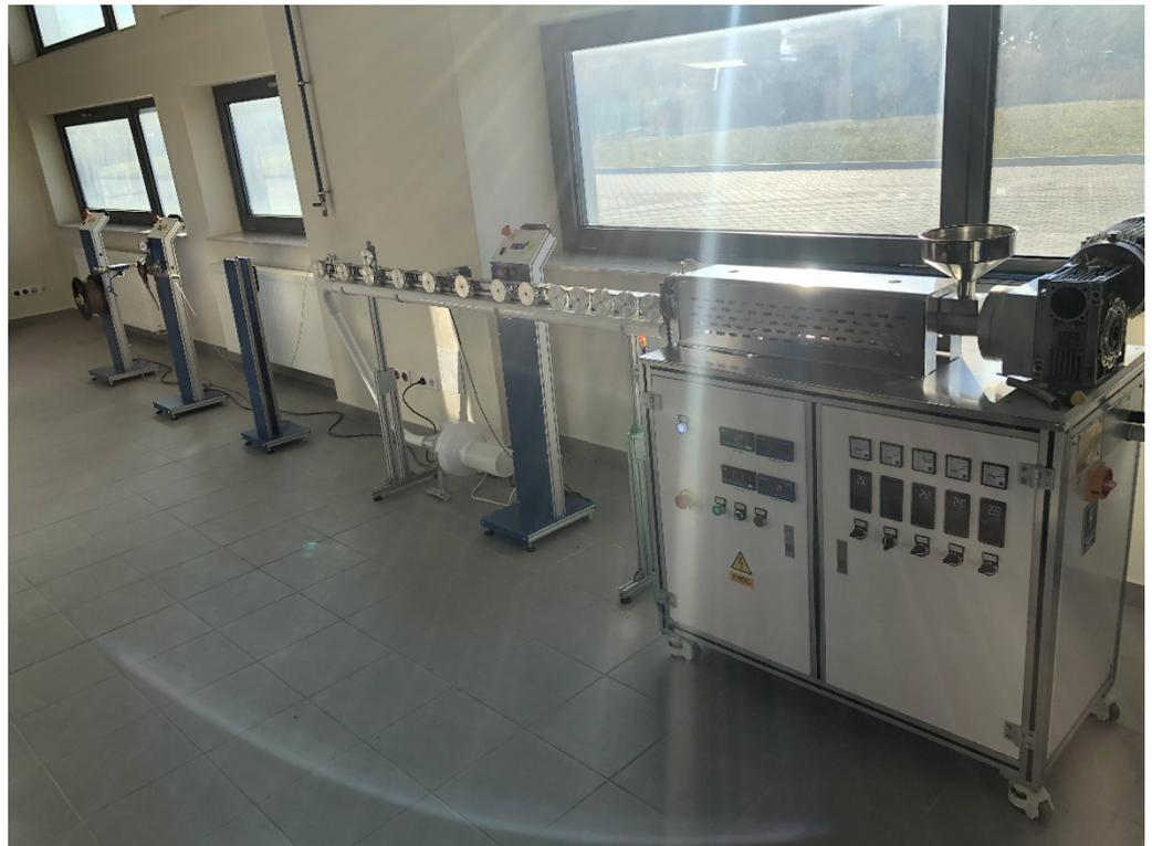
**Figure 1.** Proprietary technological line for obtaining filaments.
