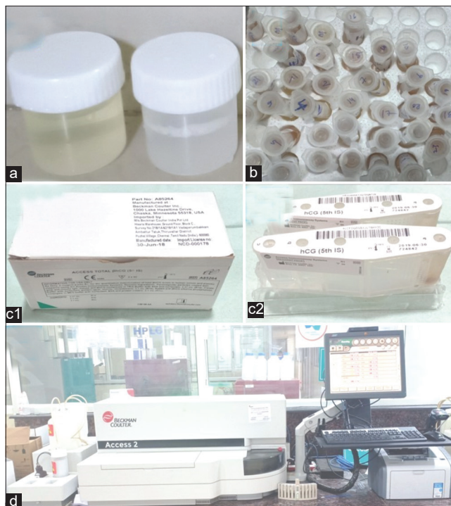
Figure 2: Evaluation of human chorionic gonadotropin- \beta in saliva and urine. (a) saliva and urine containers, (b) vials, (c1 and c2) Access human chorionic gonadotropin- \beta kit, (d) Beckman Coulter Access 2 immunoassay system
