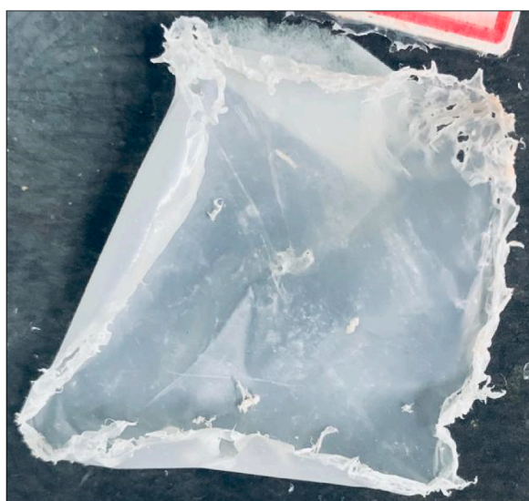
Fig. 6. A PHA film produced by B. paranthracis RSKS-3 under optimized synthetic media. A chloroform-dissolved PHA was poured into a watch glass and air-dried using a hot air oven at 60 °C temperatures.
