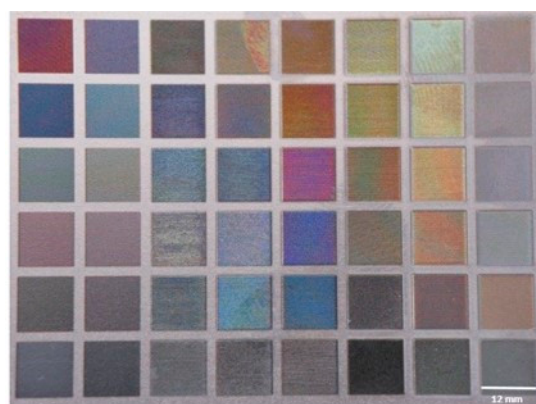
Figure 1. Palette of titanium Grade 5 surface with the sixty-four colors obtained by laser ablation (the dimensions of each single colored field are 12 × 12 mm 2 ).
