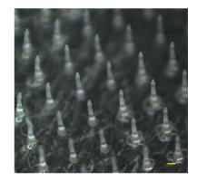
Figure 1. Micrograph of ALN(TIP)-MN (tip-ALN-loaded hyaluronic acid MN). Scale bar: 400 µm.
