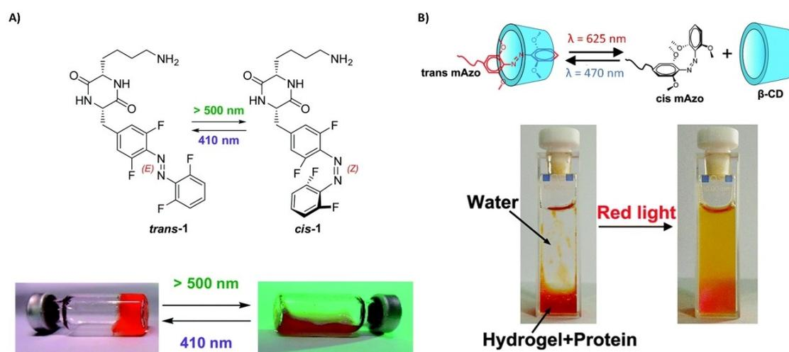
**Figure 3.** Application of red-shifted azobenzenes in photoreversible hydrogelation by A) assembly/dissociation of amphiphilic peptides; reproduced with permission from Ref. [18]. Copyright (2018) Wiley-VCH GmbH. B) complexation with  $\beta$ -cyclodextrin.<sup>[19b]</sup>
