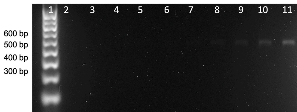
Figure 4. Gel electrophoresis of the double-tagging PCR amplification of the E. coli 16S ribosomal gene, including an initial step at 95^\circ\text{C} for 3 min followed by 25 cycles of 95^\circ\text{C} for 30 s, 58^\circ\text{C} for 30 s, 72^\circ\text{C} for 30 s, and a final step of 7 min at 72^\circ\text{C} . The amplification bands correspond to the E. coli 16S ribosomal gene (527 bp). Lane 1 is the molecular weight marker. Lane 2 corresponds to the negative control in which no DNA template has been added to the PCR mixture, while lanes 3–11 show the amplicon corresponding to DNA template concentrations at 0.1, 0.2, 0.4, 0.9, 1.8, 3.5, 7.1, 17.7, and 35.5 \text{ pg } \mu\text{L}^{-1} .
