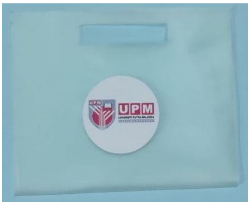
Figure 2. Corn starch (CS) with 30% sorbitol film prepared using the solution casting method.
