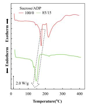
Figure 6. DSC curves of sucrose and SADP 85/15 adhesive.
