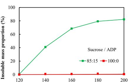
Figure 7. Insoluble mass proportion of SADP 85/15 adhesive and sucrose under different temperatures.
