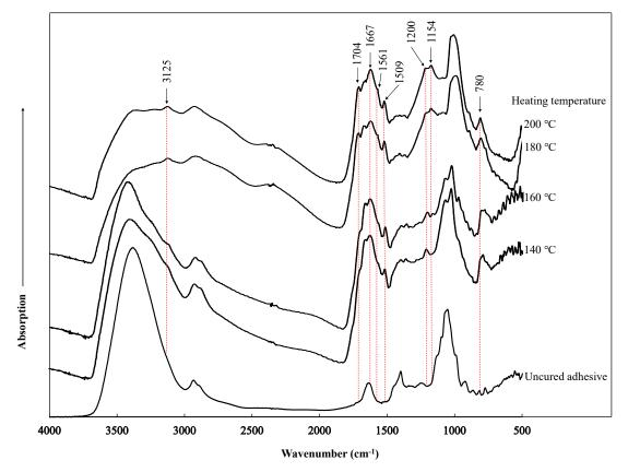
**Figure 8.** Infrared spectrum of the insoluble mass obtained from SADP 85/15 heated at different temperature and uncured adhesive obtained by drying at 80 °C for 15 h.
