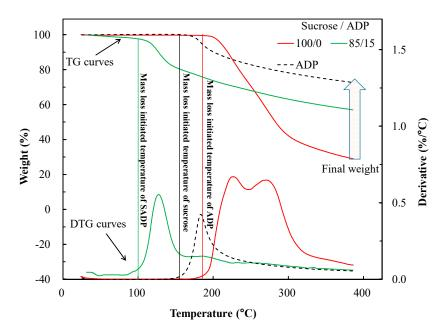
Figure 5. TG and DTG curves of sucrose (100/0), ADP (0/100), and uncured SAPD adhesive (85/15).
