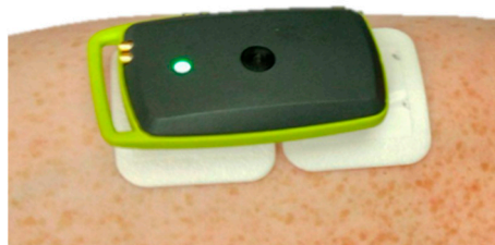
Figure 4. Electromyographic (EMG) Holter fixed to the body using Ag/AgCl electrodes.
