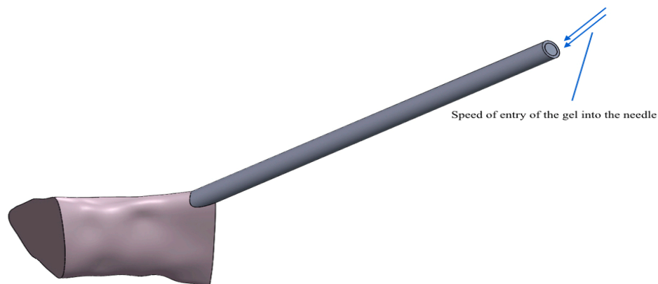
Figure 5. Indication regarding the entry speed (4 m/s) of the gel from the tank towards the needle.
