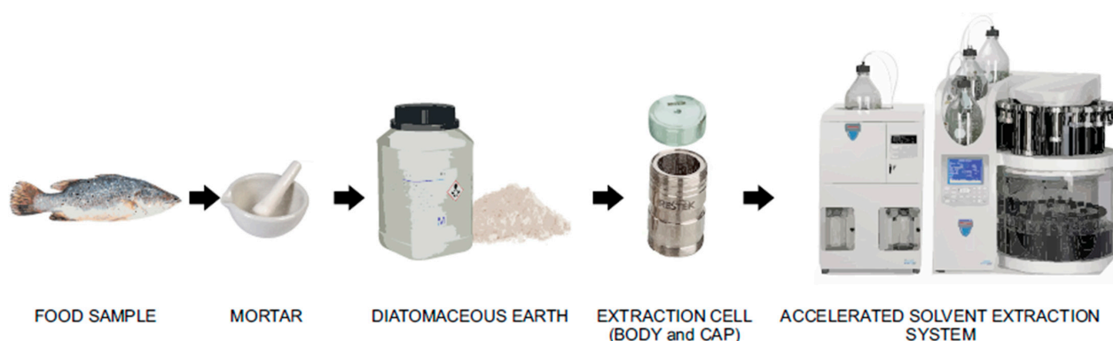
Figure 3. Flowchart of accelerated solvent extraction procedures of animal-derived food samples.
