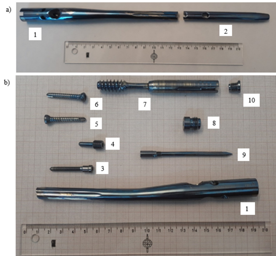
Figure 9. General view of the broken femoral nail's shaft; its proximal (1) and distal (2) parts (a) with a set of assembling parts: proximal part of the broken nail's shaft (1); blocking bolt (3); nail's screw (4); two self-tapping locking screws (5 and 6); telescopic lag screw (7); end cap (8); anti-rotation pin (9); cap (10) (b).
