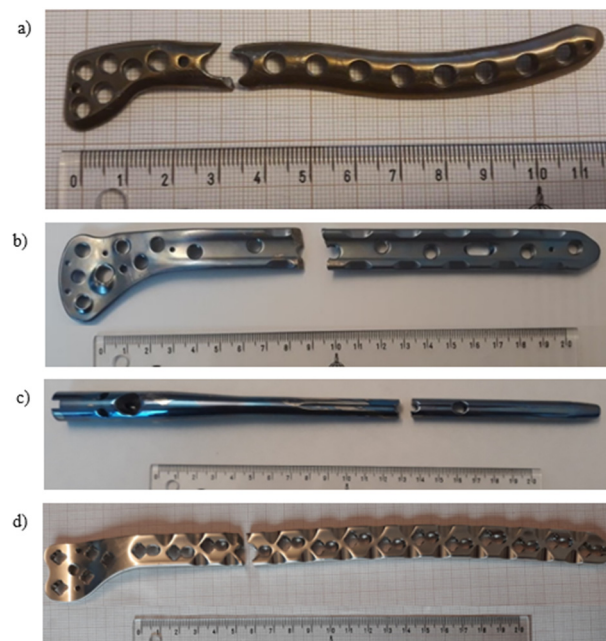
Figure 1. General view of the exploited implants with different geometries made of pure titanium clavicular (a) and distal femoral (b) plates, Ti-6Al-4V femoral gamma nail (c) and a X2CrNiMo18-14-3 femoral condylar plate (d).
