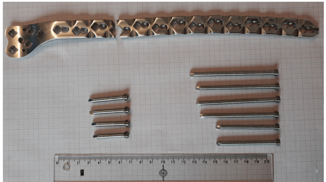
Figure 13. General view of the explanted steel femoral condylar plate.
