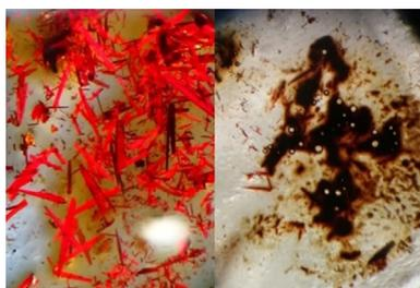
**Figure 3.** Photographs of crystals of **4b** at  $-30^\circ\text{C}$  (left) and their quick decomposition at  $-15^\circ\text{C}$  with concomitant CO evolution (right).
