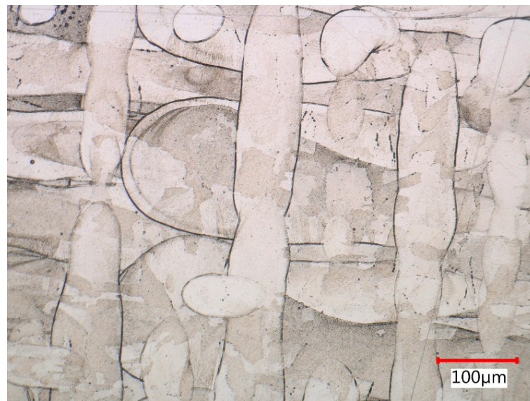
Figure 17. Solidification tracks in melting levels (oxalic etchant).
