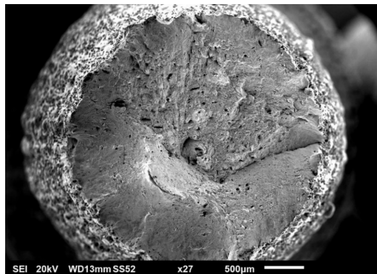
Figure 8. SEM observation, secondary electron spectrum—overall fracture morphology.
