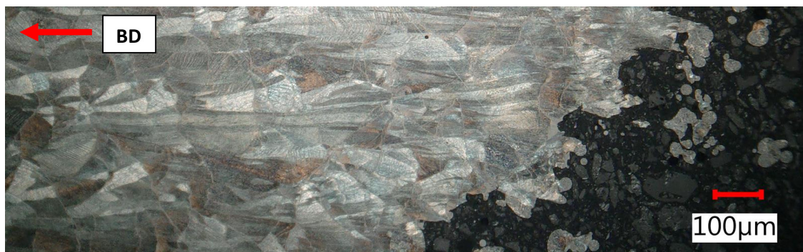
Figure 20. Elongated melt pools in close proximity of tensile fracture, as built + stress relief, lateral section.
