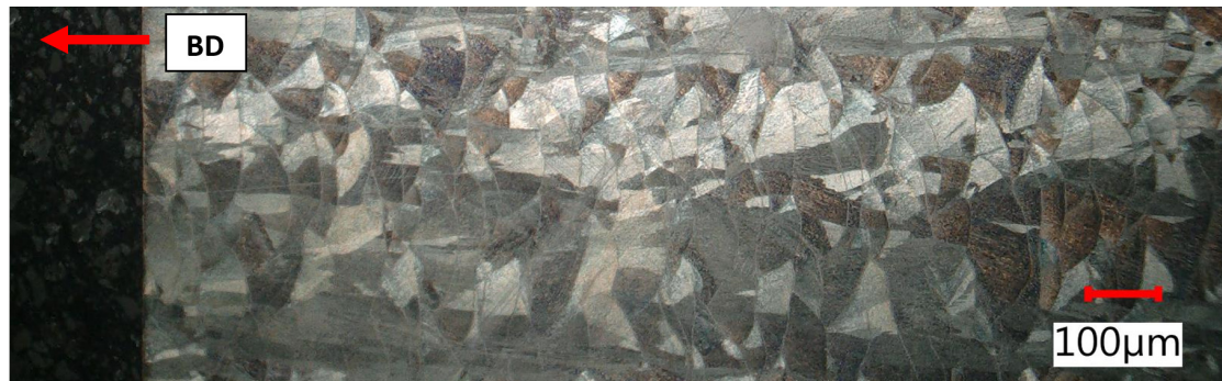
Figure 19. Undeformed clamping part area, as built + stress relief, lateral section.
