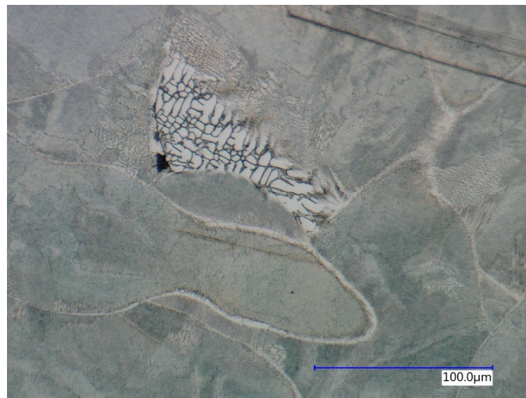
Figure 15. Dendritic solidification structure of unmelted particle.
