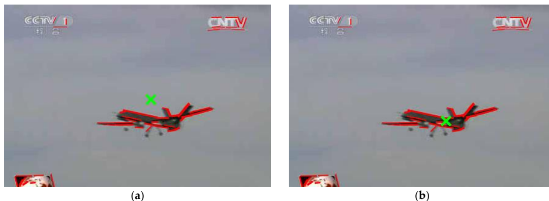
Figure 3. A comparison of the results of the methods: (a) Image moment method; (b) Mean shift algorithm.
