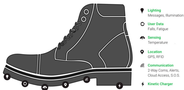
Fig. 8 Smart boots to prevent infectious viruses like COVID-19 by contact tracing, geo-fencing and social distancing alerts, source: Camas (2020)
