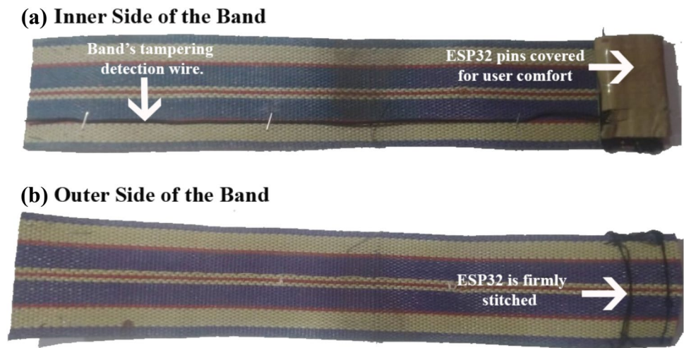
Fig. 9 IoT-Q-Band system for real-time monitoring of the health condition of individual and ensure social distancing to prevent the spread of COVID-19 virus, source: Singh et al. (2020)
