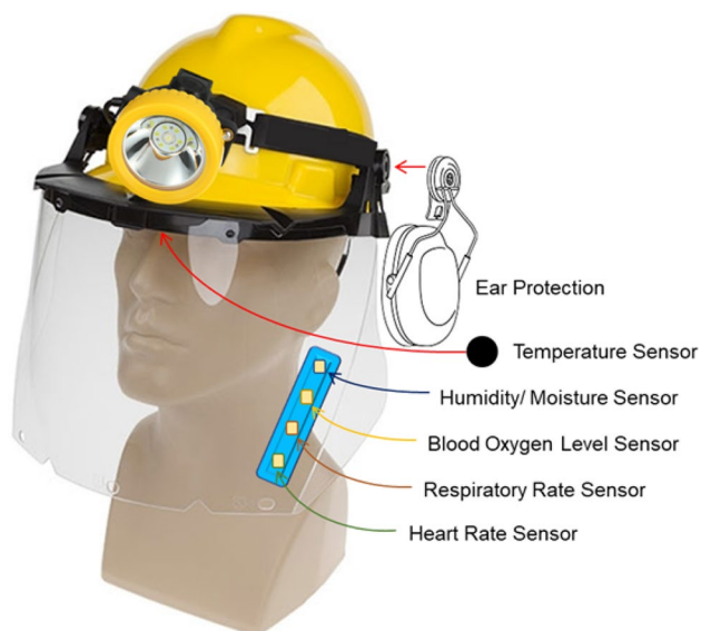
Fig. 7 Digital face shield for the mining industry to manage and control the impacts of COVID-19, source: Das (2020)
