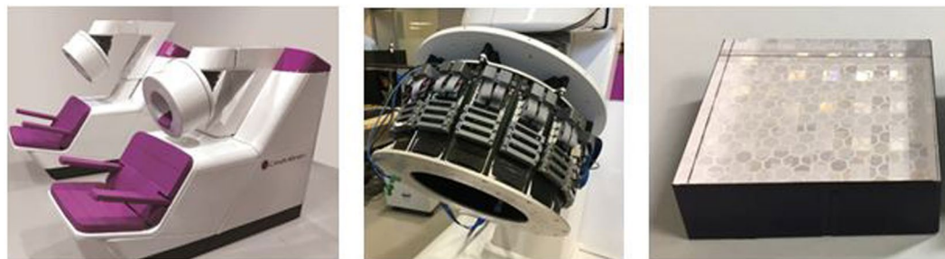
Figure 1. Image of the CareMiBrain system (left), detail of the detector electronics (center), crystal configuration (right).
