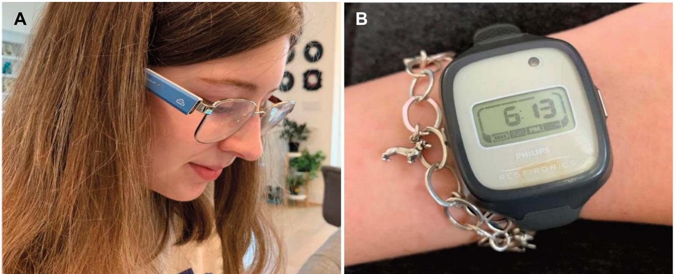
**FIGURE 1.** Wearable sensors used in this study. (A) Clouclip device fitted to the right temple of a spectacle frame in a myopic participant. (B) Actiwatch Spectrum Plus.
