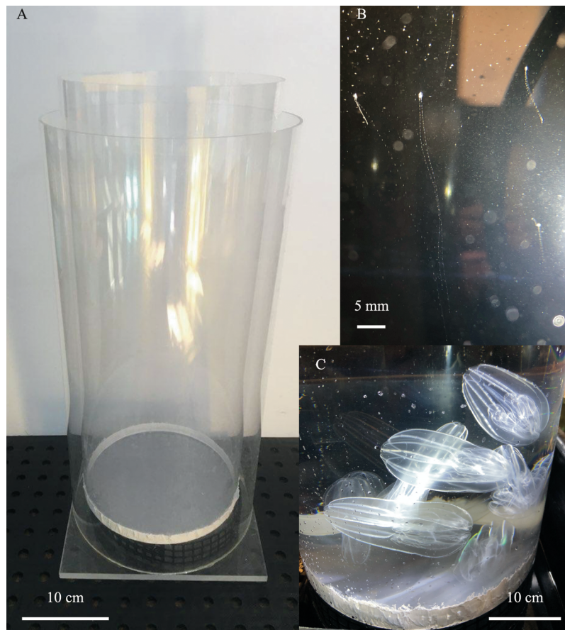
Figure 8 Shorter and wider diffusion tubes for other species of gelata. (A) 30 cm wide diffusion tubes used for Bolinopsis infundibulum and Nanomia bijuga culture, (B) larval N. bijuga at 35 days post settlement visible near the top of the tube and (C) mature B. infundibulum spawning under bright light, the wider and shorter tube makes it easier to place and remove the adult lobates.
