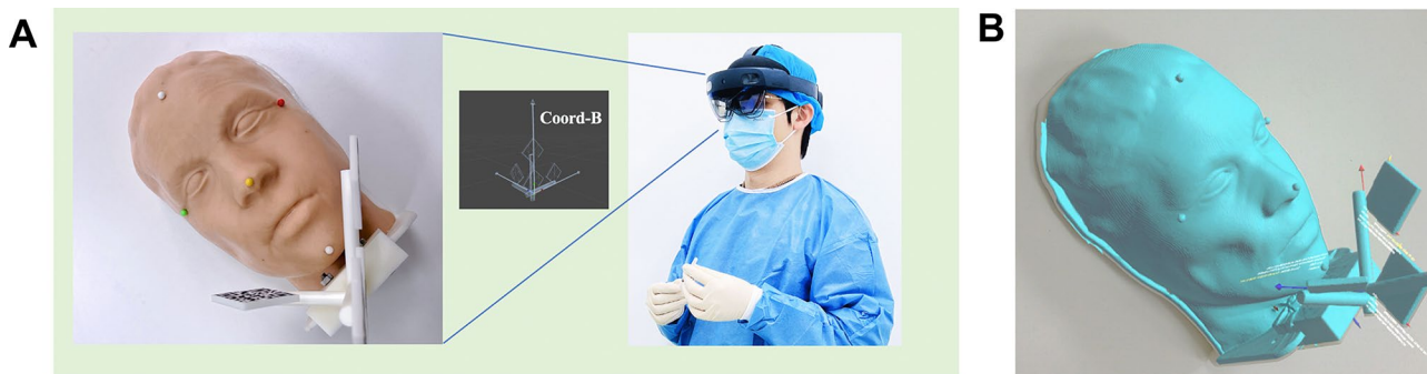
Fig. 4 Achieving Augmented Reality Fusion using Artificial Marker-based Tracking and Registration Method. A: HoloLens 2 identifies the QR codes in the real space to obtain coordinates Coord-B. B: Display of augmented reality fusion from the perspective of augmented reality
