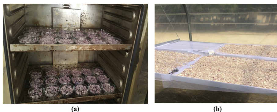
Fig. 1. (a) Photo of the pyrex cups for monitoring drying kinetics in the oven and (b) photo of a rack for monitoring drying kinetics in the solar greenhouse.
