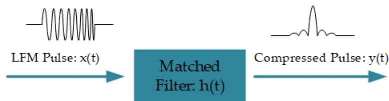
Figure 12. Pulse compression principle with linear frequency modulation (LFM, or FSP) and matched filter.
