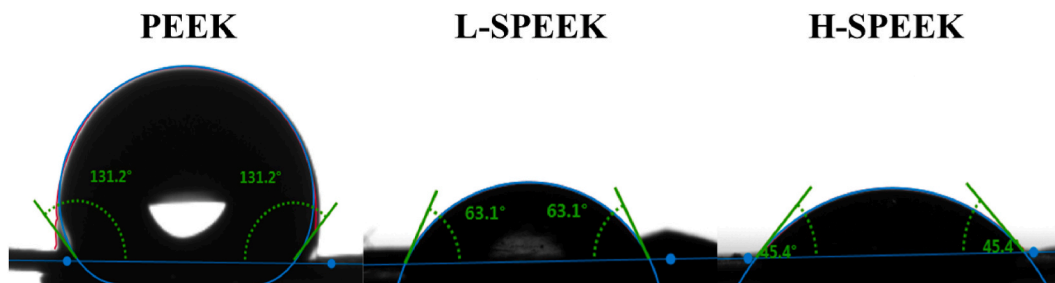
Fig. 3. The water contact angles of PEEK, L-SPEEK and H-SPEEK.
