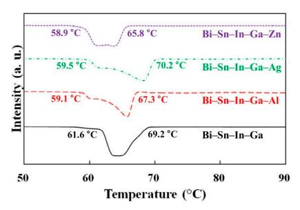
**Figure 2.** Differential Scanning Calorimetry (DSC) data from some High Entropy Alloy (HEA)-like solders, indicating the effect of the elemental composition on the melting point. Reprinted from [34], with permission from Elsevier.
