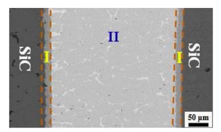
**Figure 4.** A cross section through a joint formed between two pieces of SiC, using CrFeCoNiCu alone as the filler, at 1180 °C, 60 min. (I) Denotes the reaction layers and (II) the main joint seam. Reprinted from [39], with permission from Elsevier.
