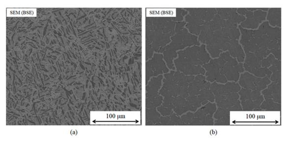
**Figure 8.** SEM (BSE) micrographs of as-cast (**a**) equiatomic NiCrFeGe, and (**b**) optimised Ni, Fe-rich, Cr-lean NiCrFeGe alloys. Significant reduction in the concentration of the dark contrast Cr,Ge-rich intermetallic phase is observed in (**b**) as compared to (**a**), resulting from the Thermo-Calc modelled composition optimization towards increased FCC solid solution molar content.
