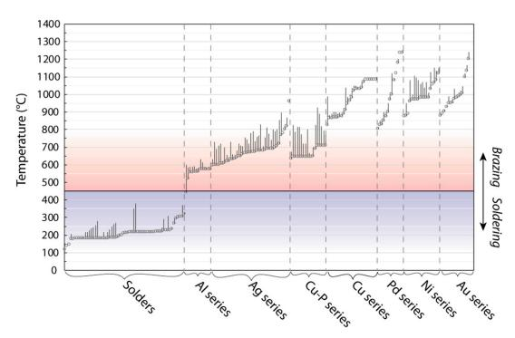
**Figure 9.** The melting characteristics of standard soldering and brazing filler metals, split into the families used in the standards. The plotted point is the solidius, and the vertical line represents the melting range until the liquidus temperature is reached. The low number of available fillers around 350–500  $^{\circ}$ C is clear. Data for brazing filler metals are from ISO: 17672 and for solders from BS EN ISO 9453.
