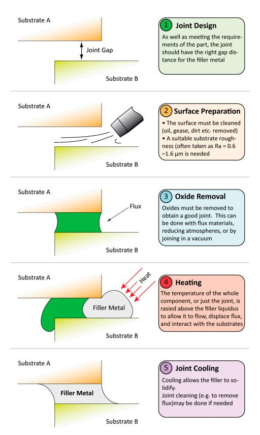
**Figure 1.** A schematic of the five main stages in joining using a filler metal process. Note that the details of these steps may vary considerably in different applications, and the pictorial representation here does not depict the details of all processes.
