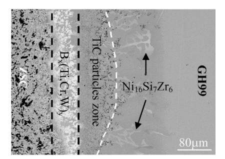
**Figure 3.** A cross section through a joint formed between ZSC and GH99 superalloy, using CrFeCoNiCu and Ti foils, at 1180 °C, 60 min. Reprinted from [35], with permission from Elsevier.
