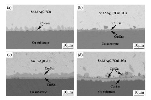
**Figure 13.** Morphologies of as-reflowed (a) Sn-Ag-Cu/Cu and (b) Sn-Ag-Cu-Ga/Cu interface, (c) Sn-Ag-Cu/Cu and (d) Sn-Ag-Cu-Ga/Cu interface aged at 180  $^{\circ}$ C for four days. Reprinted from [105], with permission from Elsevier.
