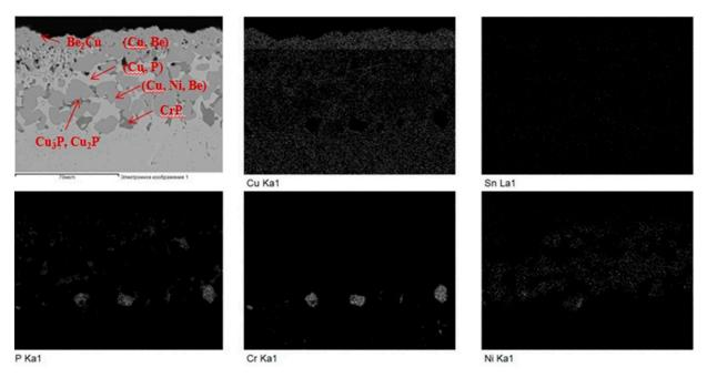
**Figure 11.** SEM image of a joint formed between Be and CuCrZr using a Cu-9.1Ni-3.6Sn-8.0P filler (STEMET 1101), and the EDS compositional maps. Many different phases are identified as indicated on the SEM image. Reprinted from [92], with permission from Elsevier.
