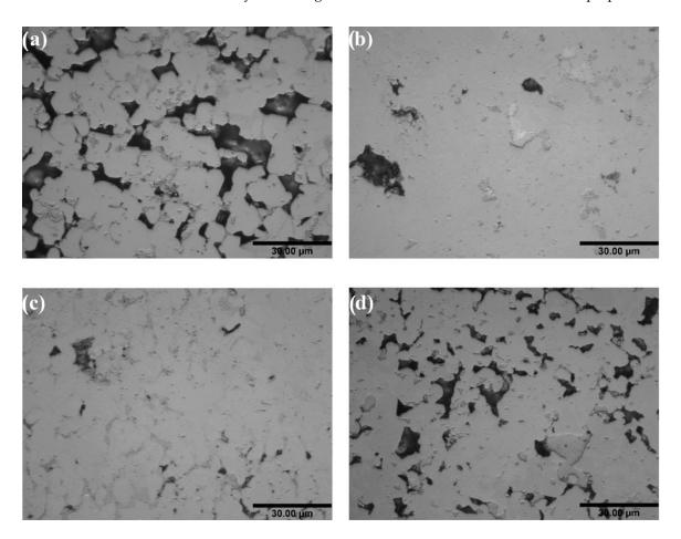
**Figure 10.** Optical micrographs of the microstructure of each of the four alloy systems at 100x magnification. ZnGaCu-(AuSn) (a), ZnGaCu-Sn (b), ZnGaCu- (AuBi) (c), and ZnGaCu-Bi (d). All four show the presence of multiple phases. Note there is also porosity as these observations of the alloys were made after initial alloying and casting, before preparation of joints.
