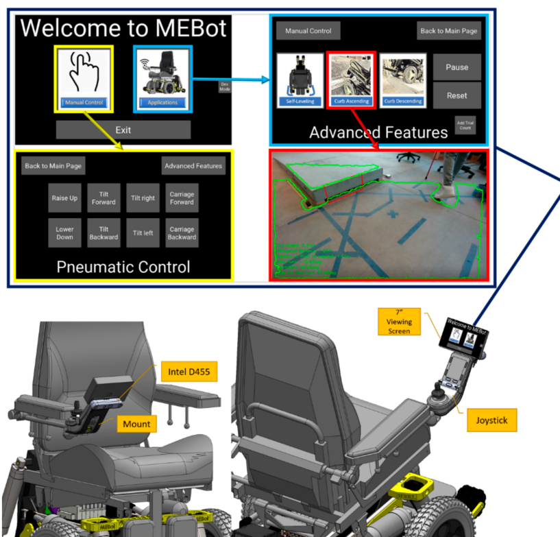
Figure 2. Intel RealSense mounts onto the wheelchair joystick and graphical user interface.
