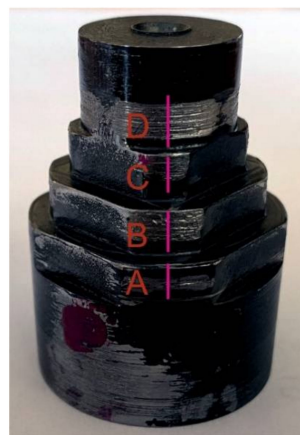
Figure 14. The sample worn initially DLC covered surfaces of steel shaft shoulders after the mating with the front planes of steel plunger fins. A, B, C, D—the worn cylindrical surfaces of the consecutive shaft shoulders.
