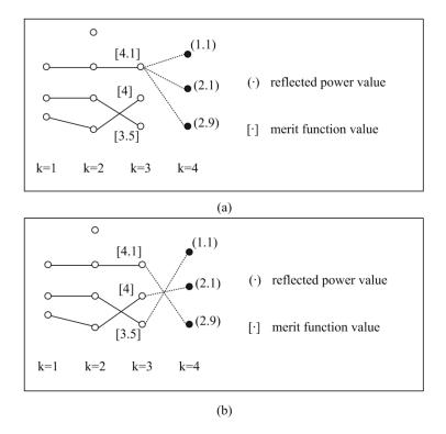
Step 4: termination and backtracking. For the final stage merit function of PDP-TBD consists of a penalty term, the threshold is difficult to be determined. In this step, a decision function is applied to replace the final stage merit function when determining the target trajectories. The decision function is a sum of reflected power. Therefore, the threshold can be determined without influence of the penalty term. For all  $\mathbf{x}_{K} \in X_{K}$ , for  $k = K, K - 1, \dots, 2$ :
