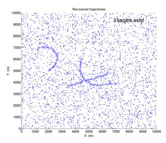
**Figure 10.** Recovered trajectories and estimated target number (Scenario-3, "-o-" represents the recovered trajectories of the targets, "·" represents the measurements).
