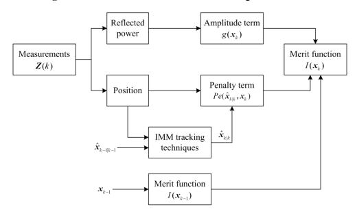
Figure 1. Merit function calculation block diagram at scan k.
