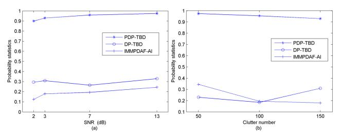
Inspection of Figure 8 and Table 2 shows that PDP-TBD is efficient to detect and track multiple maneuvering targets in this scenario, while DP-TBD and IMMPDAF-AI actually fail to detect the two targets in Scenario 2.
