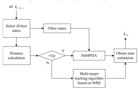
Figure 4. Tracking techniques block diagram.
