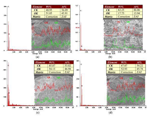
**Figure 2.** The EDAX (Energy Dispersive X-ray Analysis) wire images: (**a**) Arboblend V2 Nature, (**b**) Arbofill Fichte, (**c**) Arboblend V2 Nature reinforced with Extrudr BDP "Pearl", (**d**) Fiber Wood.
