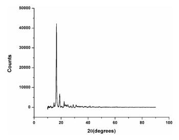
Figure 3. XRD analyses for Arboblend V2 Nature reinforced with Extrudr BDP "Pearl" material.
