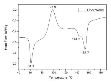
Figure 7. Highlighting the main thermal behavior of the Fiber Wood wire.
