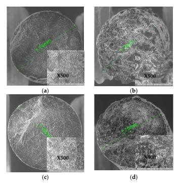
**Figure 1.** The SEM wires images: (**a**) Arboblend V2 Nature, (**b**) Arbofill Fichte, (**c**) Arboblend V2 Nature reinforced with Extrudr BDP "Pearl", (**d**) Fiber Wood.
