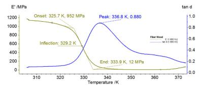
Figure 9. DMA thermogram recorded during fiber wood heating.
