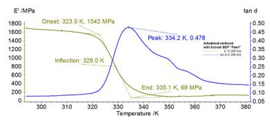
**Figure 8.** Dynamic Mechanical Analysis (DMA) thermogram recorded during heating of Arboblend V2 Nature reinforced with Extrudr BDP "Pearl".
