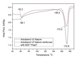
**Figure 5.** Highlighting the main thermal behavior of the wires made from Arboblend V2 Nature and Arboblend V2 Nature reinforced with Extrudr BDP "Pearl".
