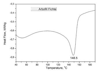
Figure 6. Highlighting the main thermal behavior of the wire made from Arbofill Fichte.
