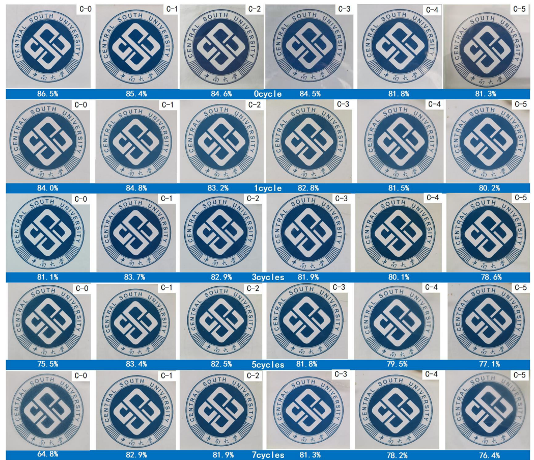
Figure 10. Digital photos and light transmittance of samples at different aging cycles.
