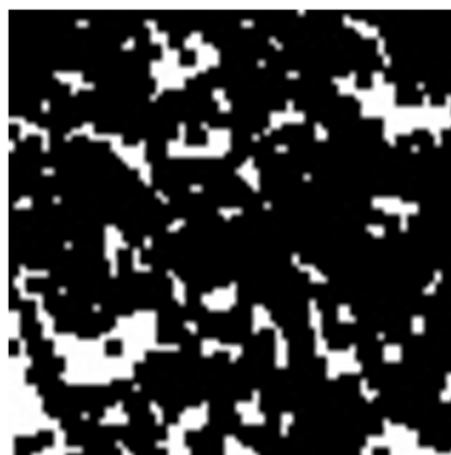
(c) Binarized image (threshold value 100): Black ratio = 82.7%
