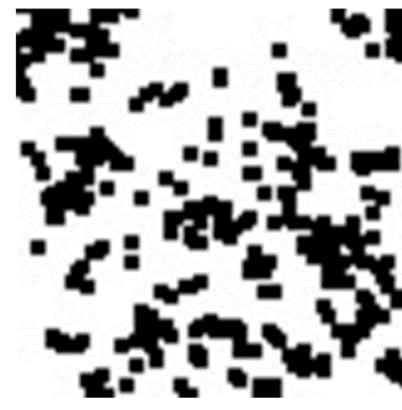
(d) Binarized image (threshold value 25): Black ratio = 19.1%
